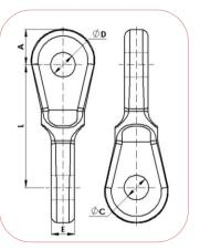
Material: Forged steel EN-10083 equivalent to ASTM A576. Steel parts finish: Hot dip galvanizing CSA-G164 / ASTM A153.
