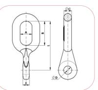
Material: Forged steel EN-10083 equivalent to ASTM A576. Steel parts finish: Hot dip galvanizing CSA-G164 / ASTM A153.
