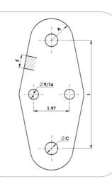
Material: Steel plate EN-10025 equivalent to ASTM A36 or ASTM A572. Steel Parts finish: Hot dip galvanizing CSA-G164 / ASTM A153.
