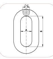
Material: Forged steel EN-10083 equivalent to ASTM A576. Steel parts finish: Hot dip galvanizing CSA-G164 / ASTM A153.
