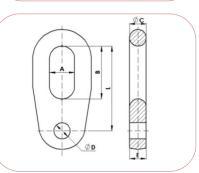
Material: Forged steel EN-10083 equivalent to ASTM A576. Steel parts finish: Hot dip galvanizing CSA-G164 / ASTM A153.
