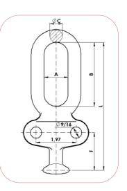
Material: Forged steel EN-10083 equivalent to ASTM A576. Steel parts finish: Hot dip galvanizing CSA-G164 / ASTM A153.
